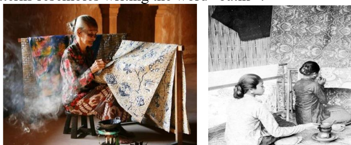
Figure 1. Hand-drawn batik, created using hot wax, a canting tool, and cloth, typically done while sitting on a bench or the floor
