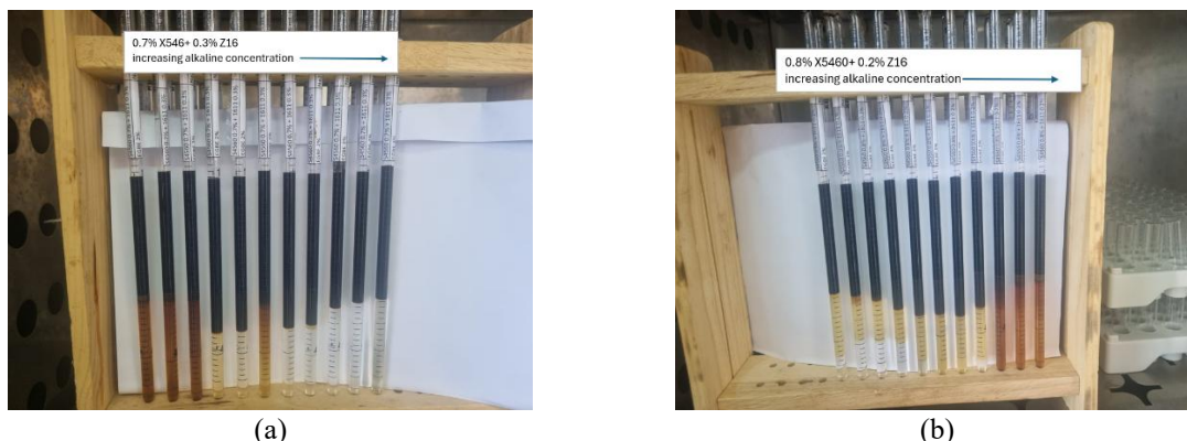
Figure 4. Salinity Scan Result on Seventh Day of 0.7% X546 and 0.3% Z16 (a); 0.8% X546 and 0.2% Z16 (b)
