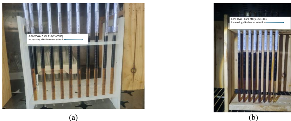
Figure 5. Salinity Scan Result on Seventh Day of 0.6% X546 and 0.4% Z16 Before Adding EGBE Concentration and Salinity Range (a); 0.6% X546 and 0.4% Z16 After Adding EGBE Concentration and Salinity Range (2.7%–3.4%) (b)
